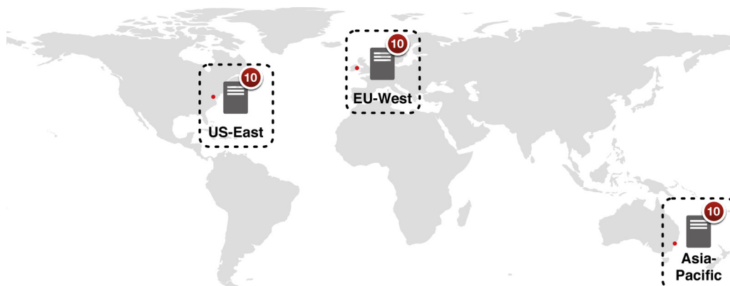
Fig. 2. The distributed pre-study with 30 nodes on Amazon EC2. (For the centralized pre-study, 30 nodes were deployed in the region US-East.)
